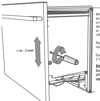
With the front panels fitted, insert an appropriately sized Philips screwdriver into the hole above the door pin and rotate the panels up or down to align the gaps in your cabinetry.
